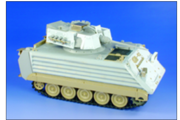
look close to the real one. Finely woven mesh screens were added to the engine deck.
